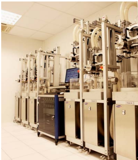
Source CARMAT – Endurance test room for complete systems, can accommodate up to 12 systems in a controlled environment.
