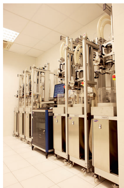
Source CARMAT - Full system endurance test room, which can host up to 12 systems in a controlled environment.
